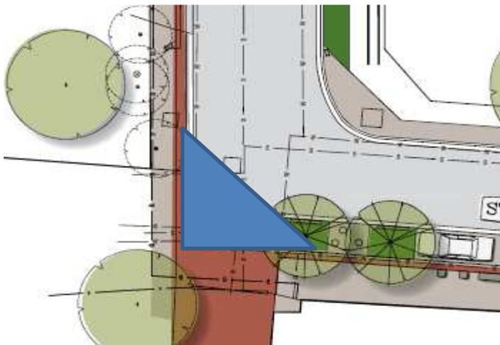
No detail is given for the road design south of the Faulding Building, including whether the shared zone/ space concept extends south of Reid Street. The design does not appear to incorporate a large protuberance that currently exists at Reid Street. Nor is detail given on the threshold treatment to highlight or demarcate the shared zone/space, which should be an important
