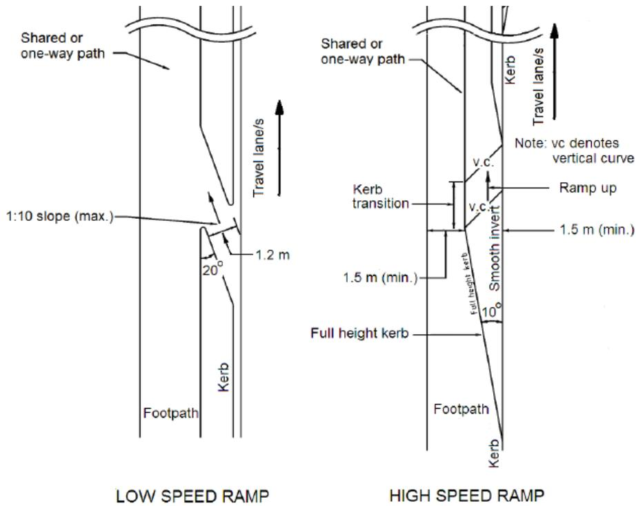
As the path is bike-only, pedestrian use would be low. While the proposed situation is not identical to the guidance situation, Figure 4.10 shows that a kerb ramp for low speed exit from a road should be aligned at an angle of some 20 degrees to the roadway.
