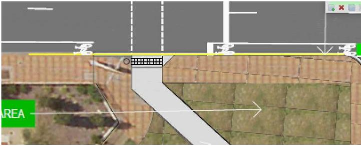
As shown, the bike path proceeds to the PAC entry in a contrasting pavement to the footpath, however there is no separate area for pedestrians to wait and cross. We would like to see a separate pedestrian crosswalk to the east of the bicycle crosswalk (which should be controlled with a bike lantern to permit cyclists to ride across). This would minimise pedestrian/ cyclist conflict on the northern footpath.
