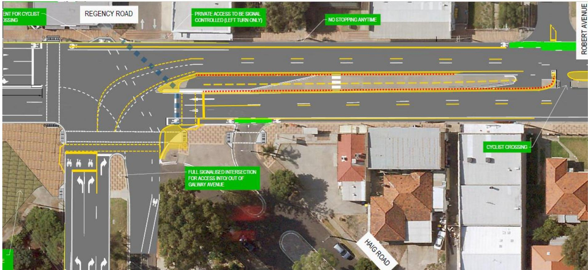
Yellow = new kerbs and line-marking, compared to option 1 or option 2 concepts (which have been combined to create the above sketch)
