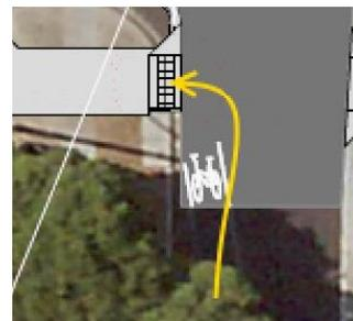
For Galway Terrace, this isn’t as bad as at other places (as long as a cyclist doesn’t follow the line of the bike lane), because the bike lane is slightly away from the kerb. However, the swinging out would occur at the same point where left-turning cars are wanting to tend to the left, and drivers would not expect a cyclist to veer into their path of travel. This creates a conflict between motorist and cyclist travel paths, with little opportunity for either party to manage this.
