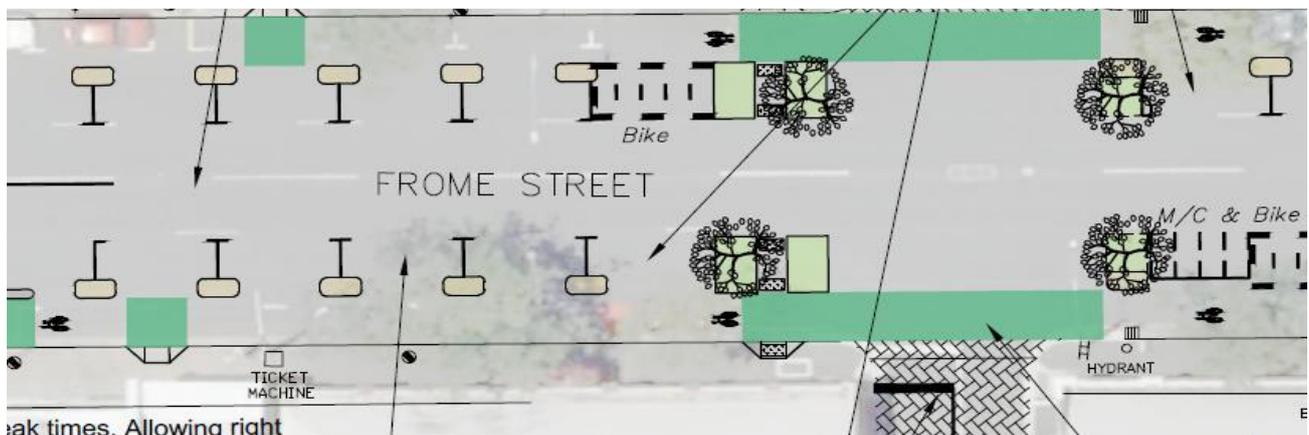
This concept showed a separator between the bike lane and parking, which widened out next to side streets to accommodate trees. One complaint about the existing Frome Bikeway is that this did not occur and the landscaping areas were not constructed to allow trees to be planted at a later date.
