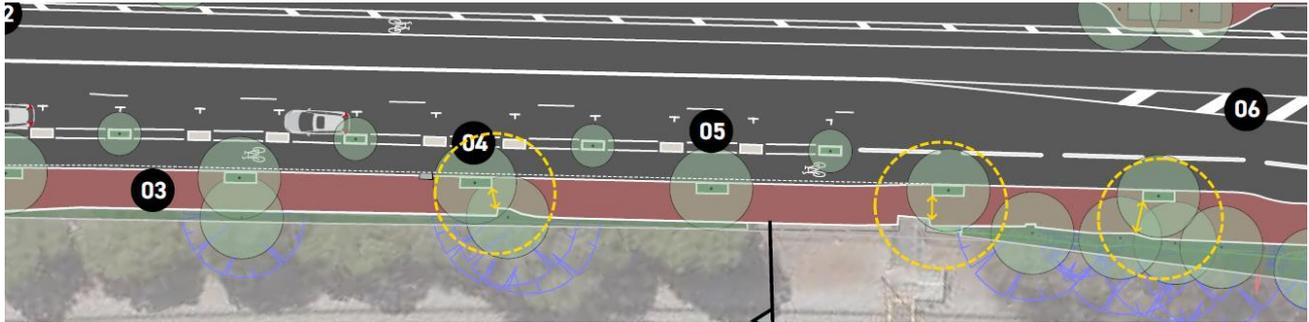
As noted for section A, the western separated bike lane could be reduced from 2.5m to 2.4m as long as the kerb to the footpath and the separator both have laid-back rather than upright profiles.
