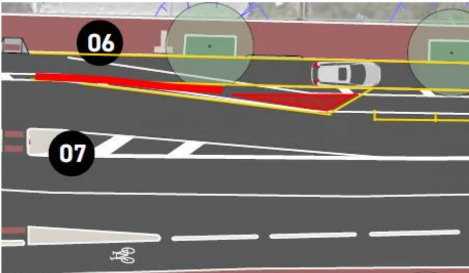
From Austroads, a buffer ('safety strip') between parallel parking and a general bicycle lane should be 0.4-1.0m wide, as follows.
