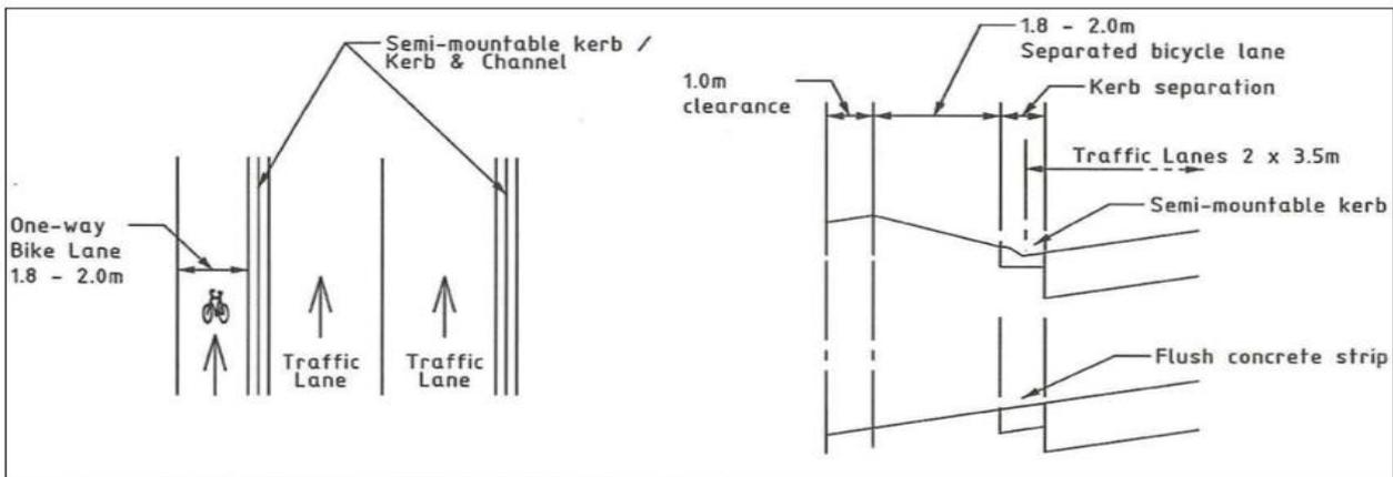
Note: A one-way crossfall should be applied where a flush concrete strip is used so that drainage does not accumulate on the bicycle path.
